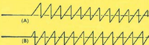
WAVE FORM AT POINT X (FIG. 5) AT START OF OSCILLATION. (A) WITHOUT BIASING RESISTORS R3 AND R4. (B) WITH BIASING RESISTORS R3 AND R4
