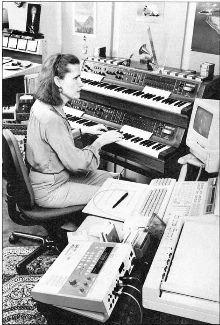
Now how perfect is that perfect fifth? Carlos playing a Synergy, flanked by computer gear (clockwise from center): two Synergys, Apple Macintosh, Hewlett-Packard computer, Mac keyboard and numeric keypad, graphics tablet, Hewlett-Packard plotter, Roland SBX-80 sync box.
